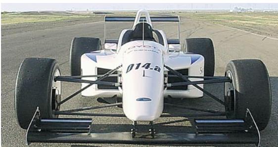
Figure 5: In order to improve cooling, intake area was increased to reduce duct losses.
