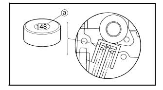
ADJUSTING THE VALVE CLEARANCE
