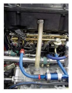
Fig. 13.3 Fuel-injection system showing injectors (red wires attached), fuel rails, dump valve (to right of centre), and engine breather discharging to airbox.
