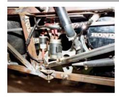
Fig. 13.2 Fuel pump and filter for carburettor setup.
