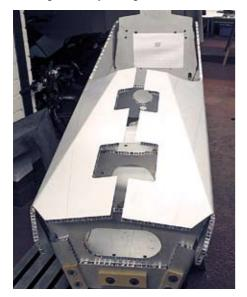
Fig. 8.12 Dummy run of monocoque folding.
