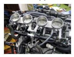
Fig. 13.4 Fuel-injection throttle bodies.
