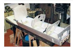
Fig. 8.11 'Dry' fitting of bulkheads.
