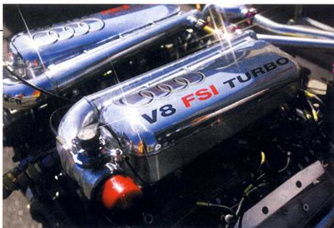
Twin polished plenums highlight an intake system designed to maximize power output despite a pair of 32.4-mm (1.28-in) intake restrictors and a 24.2-psi (167-kPa) turbo boost limit.
