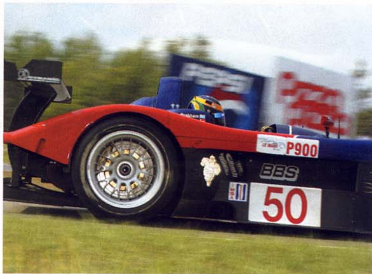
The LMP-01's massive six-piston AP brake caliper clamping the 15.0-in (380-mm) carbon-fiber disc is clearly visible through the spokes of the 18-in BBS wheel.
