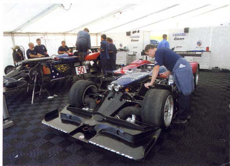
With its front bodywork removed, the front underwing of the Panoz LMP-01 is plainly visible. The twin nostrils at the top of the tub are the air restrictors leading to the car's unconventional front-mounted engine.
