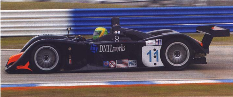
The MG-powered Lola LMP 675 car might prove to be the ideal compromise between weight and power.
