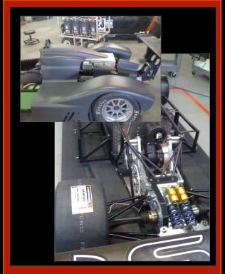
Batteries encased in chrome moly, tig welded steel structure, integral to chassis
