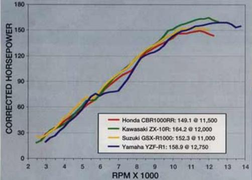
By virtue of its 5-valve-per-cylinder head design, Yamaha's 998cc R1 motor bypasses the curious set of rules which impose intake restrictions upon engines with 4 valves or less. Beyond this, the R1 mill relies on heavy doses of trickle-down MotoGP and F1 technology such as titanium valve train, ultra-lightweight camshafts and reciprocating bits, as well as cylinder-wall oil cooling and other techno-trickery to develop nearly 160 horsepower to the ground—bone stock and with a warranty!
