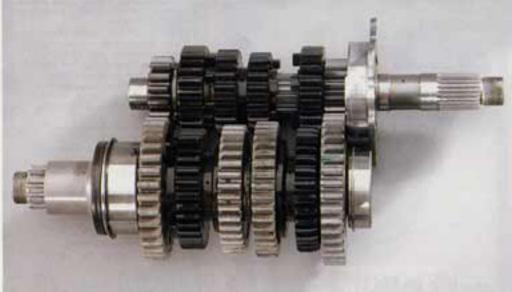
In addition to bringing high doses of highrevving, reliable horsepower, lightweight and low cost to the party, motorcycle powerplants offer the added benefit of cassette-type, sequential 6-speed transmissions that allow for quick and easy ratio changes.
