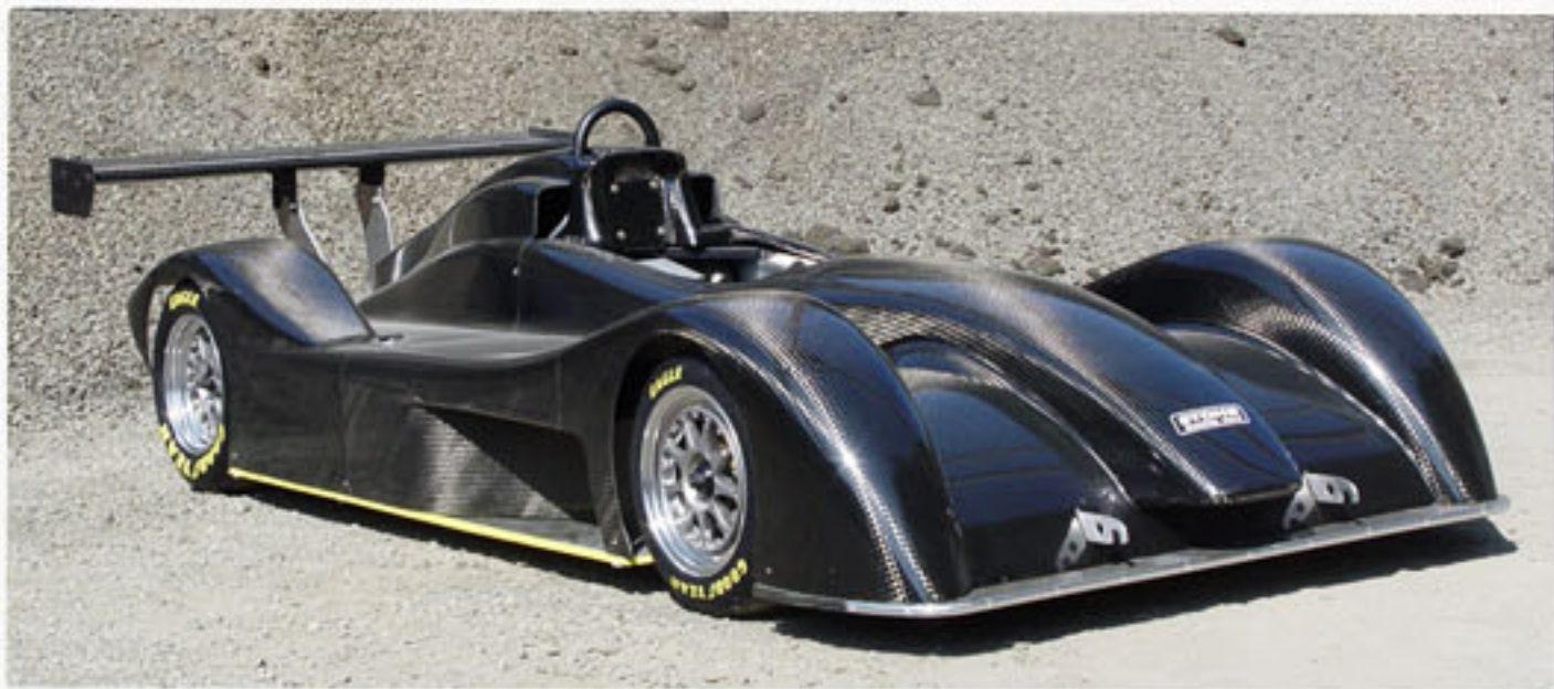
DSR which uses a part steel, part carbon fibre construction. Here with carbon body
